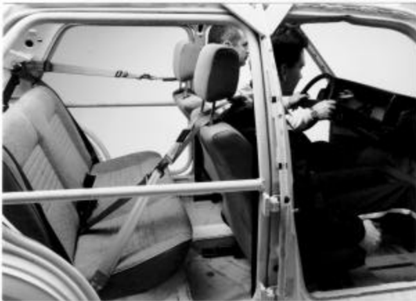
Only the passenger seat is equipped with a SCHROTH Rallye 4 harnessbelt system!
